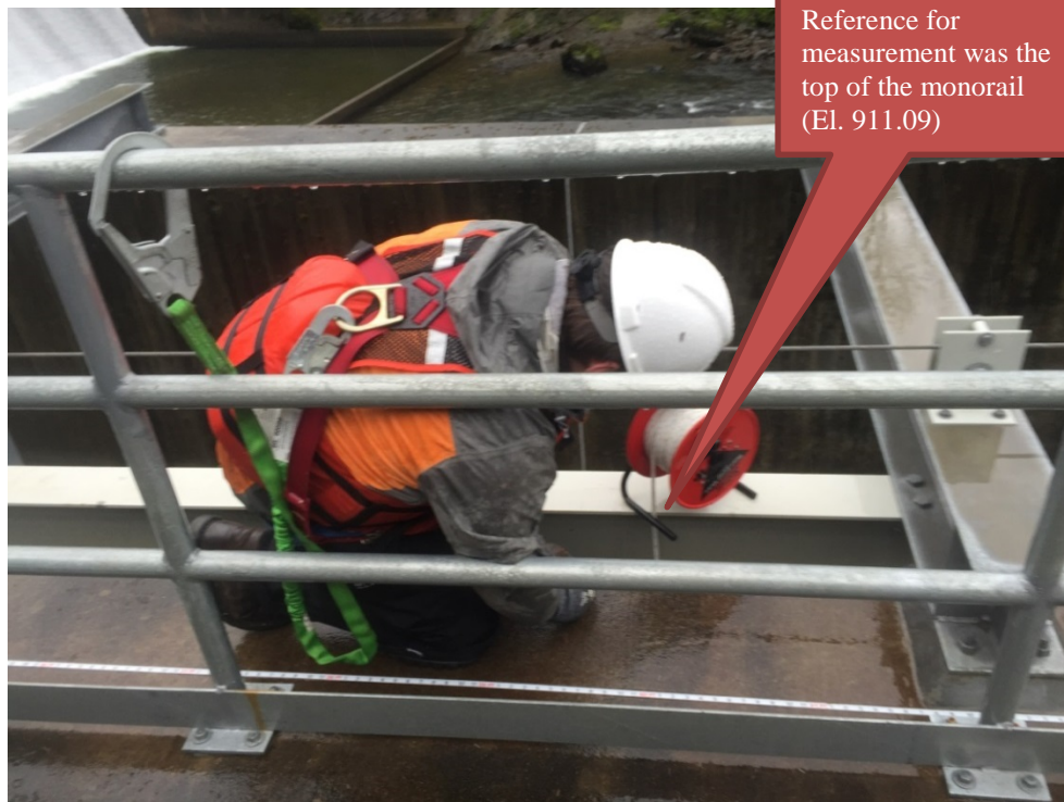
Photo 13 Water Level Measurements in the Channel
