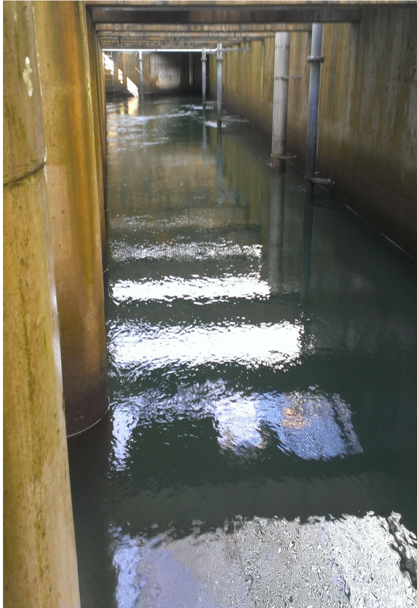
Photo 22 Flow Behind the Screens and Baffles (Screened Water Basin), Final Configuration ( Q = 210 cfs)
