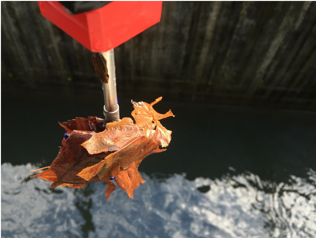
Photo 15 Bigleaf Maple Debris Loading on an ADV
