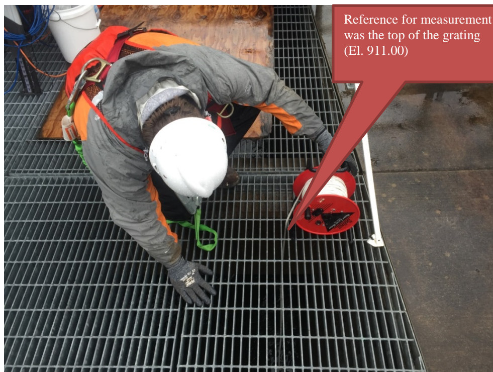
Photo 14 Water Level Measurements Behind the Vane Baffles
