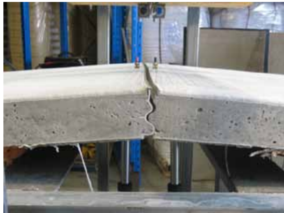
Figure 12: PLJ100 Joint cross-section at 112 mm uplift.
