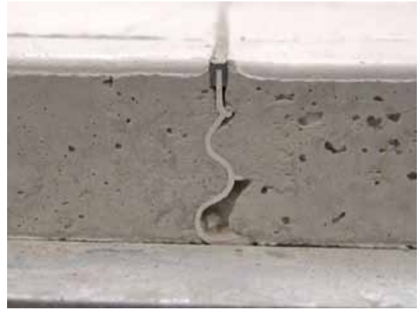
Figure 14: Cross-section Side 2 after return to zero position.
