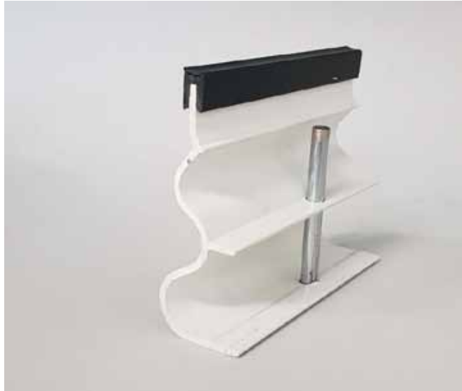
Figure 1: A sample of the PLJ100 joint consisting of a white PVC extrusion with a fitted black rubber capping strip and steel fixing pin.
