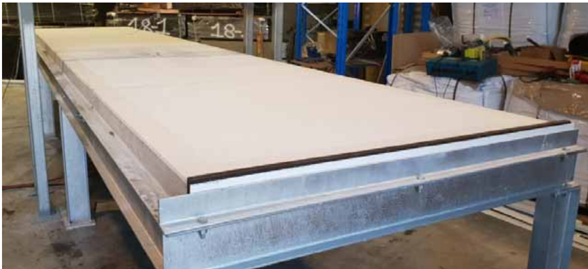
Figure 4: The test pavement was left to cure for seven (7) days.
