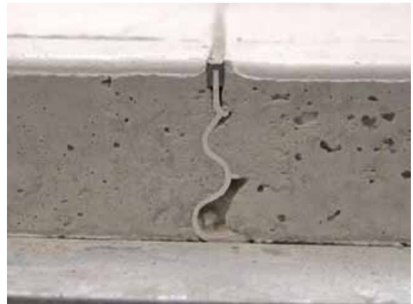
Figure 14: Cross-section Side 2 after return to zero position.
