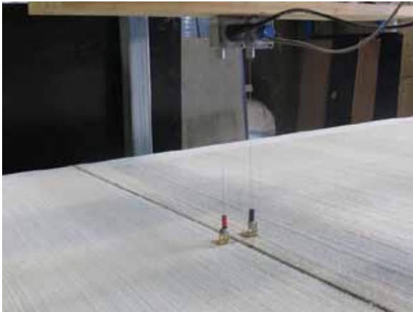
Figure 7: String pot displacement transducers attached to the pavement surface at the test joint.
