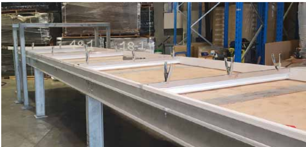
Figure 2: The steel framed test bed prior to pouring of the concrete pavement.
