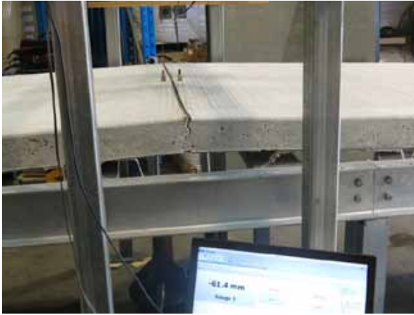
Figure 9: The pavement at 61 mm uplift displacement.
