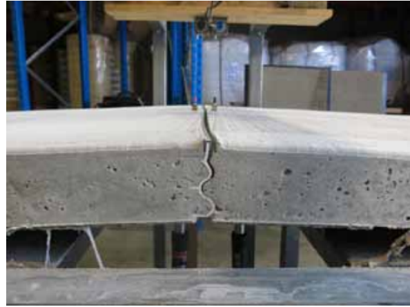
Figure 10: PLJ100 Joint cross-section at 61 mm uplift.
