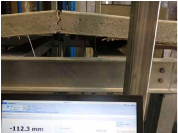
Figure 11: The pavement at 112 mm uplift displacement.
