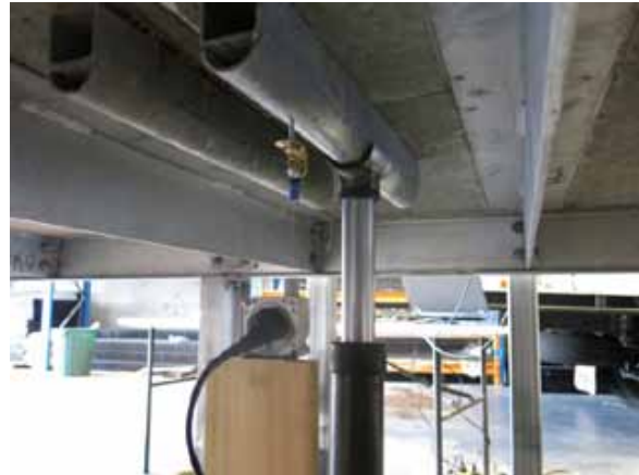
Figure 8: One string pot displacement transducer was attached below the test joint adjacent to the hydraulic ram.
