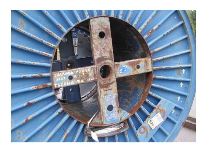
Two (2) locking pin holes 1.5" diameter Two (2) locking pin holes 2.5" diameter
