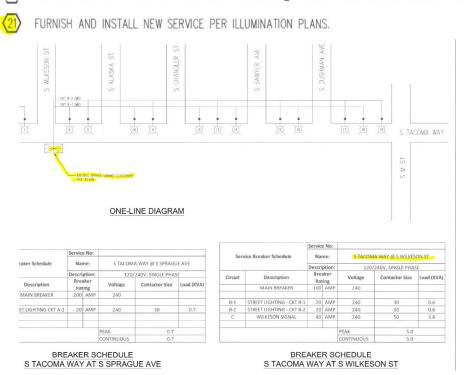
Answer 1: The plans are asking for a new service not a new service cabinet. The intent is to reuse the cabinet and install new circuits per sheet IL-1.08.
