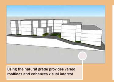
This diagram depicts a site plan that locates the primary entrance where grade change is minimal and the buildings reflect natural topography. 02 Combine complementary site features such as outdoor seating, stair climbs, accessible routes, and open space with any terracing.
