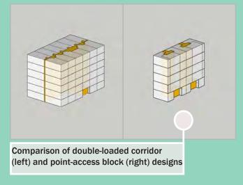
Single-stair or point-access block design provides greater opportunities for cross-ventilation and reduces reliance on mechanical cooling. 03 Employ solar, wind, geothermal, heat recovery systems, district energy, or other methods and technologies as a means to reduce reliance on offsite energy sources.
