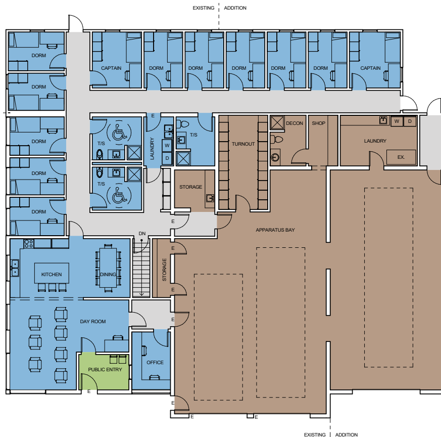
Figure 48. Floor plan of Station 4 first floor renovation and addition
