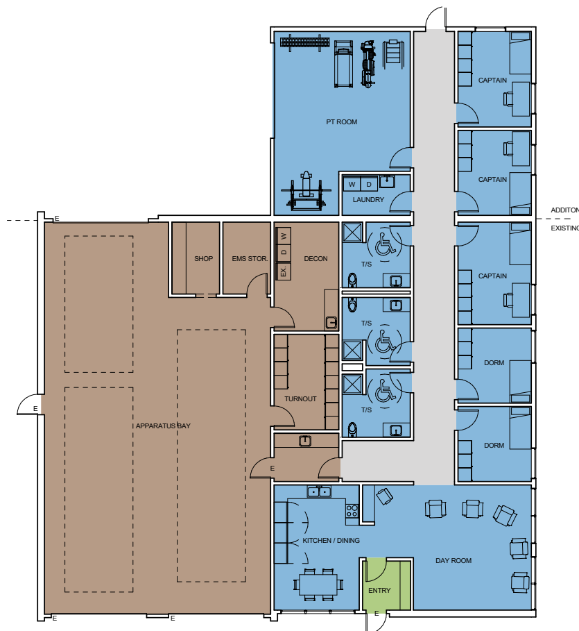
Figure 49. Floor plan of Station 6 renovation and addition
