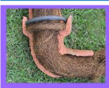
Tree roots are a common cause of clogged side-sewer lines. Roots can easily penetrate pipes through means of cracks, defects and connection joints.
