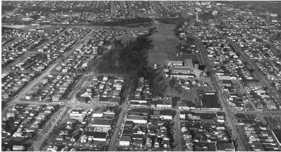
Figure A-13: 1961 aerial photo of the Lincoln District, looking north from above South 40 th St. The gulch north of South 38 th Street is cleared of brush and ready to receive fill from nearby freeway construction.
