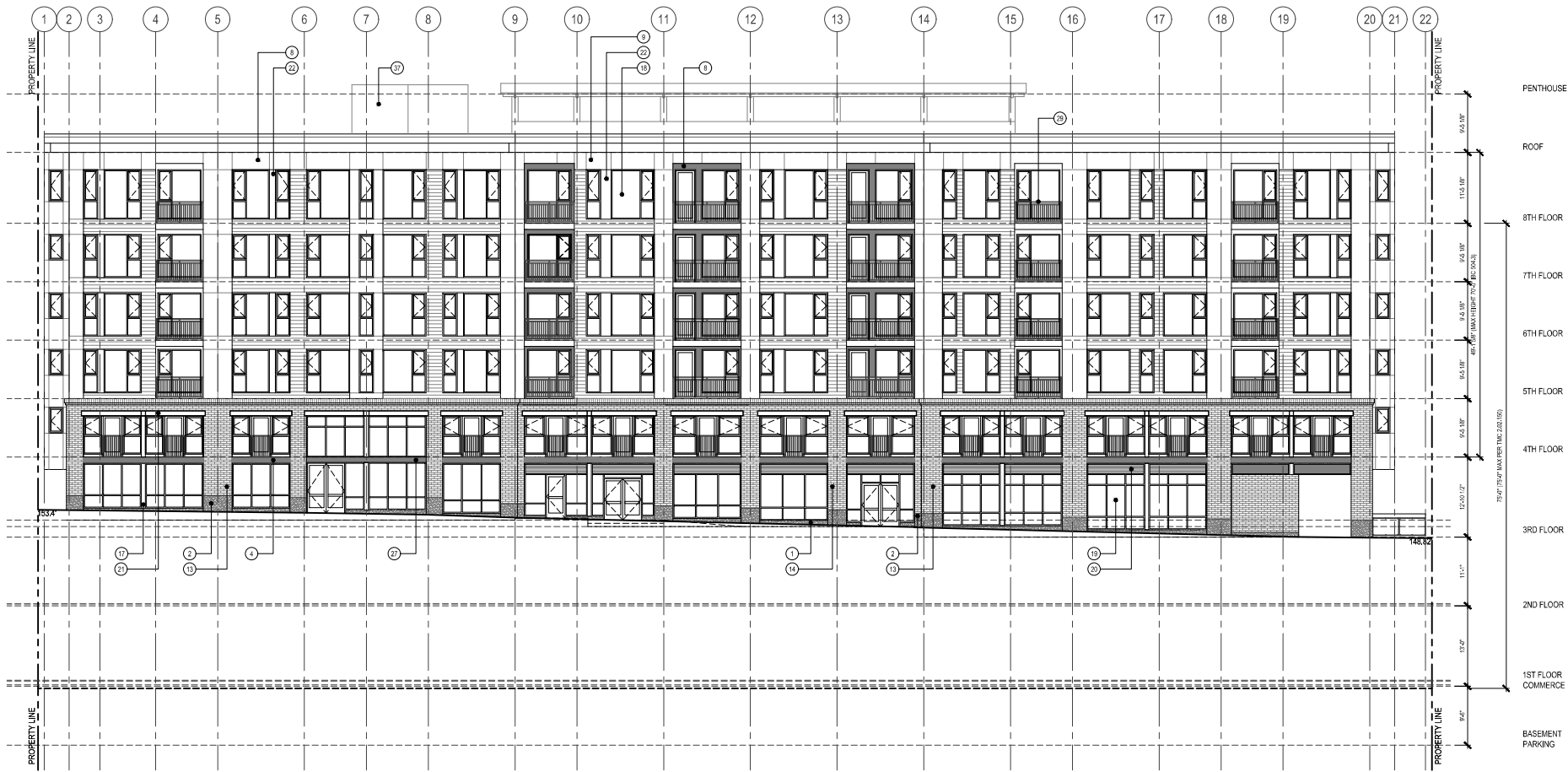
1 BUILDING ELEVATION - WEST - BROADWAY SCALE: 1/8" = 1'-0"
