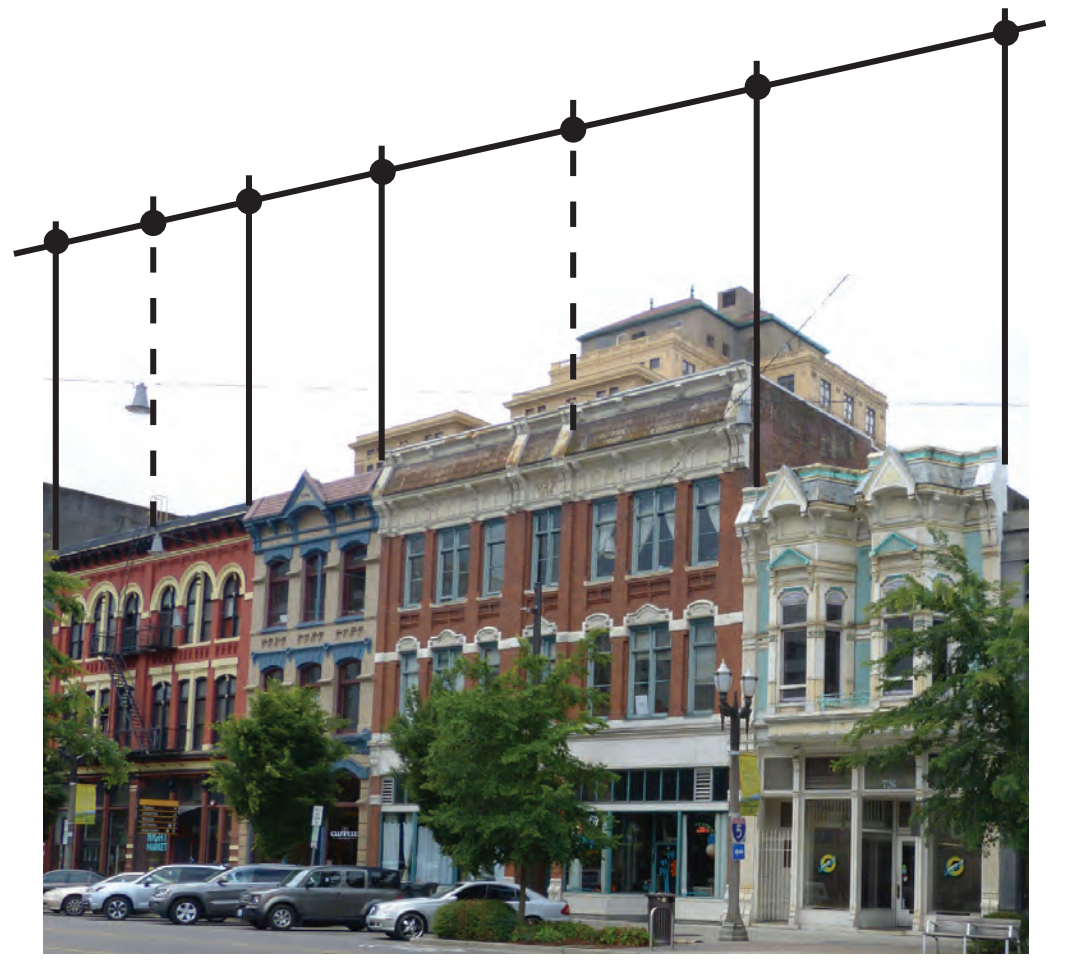
Design a new building to reflect the traditional building widths of adjacent buildings.
