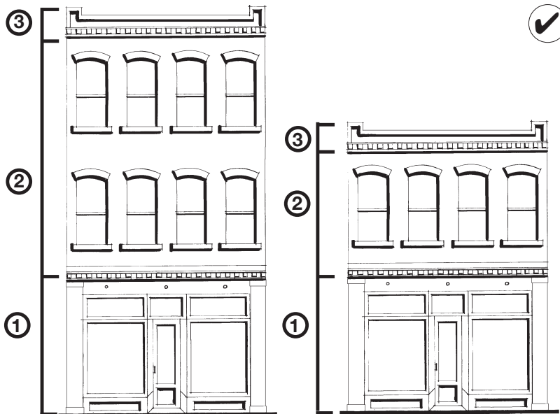
Incorporate a base, middle and a cap in the design of a new building to reinforce the visual continuity of the district: (1) base, (2) middle and (3) cap.
