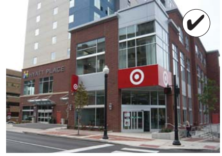
Vary the height of the new building along the street wall so that it does not read as one large, static mass.
