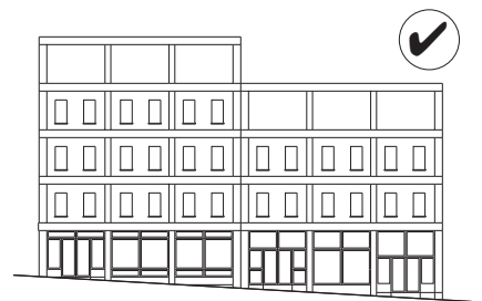
When designing a new building for a site with a sloping topography, step the building to maintain a constant street presence.
