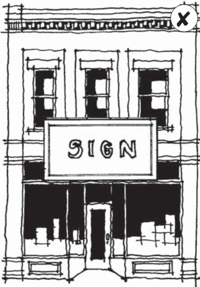
Locate a sign such that it does not obscure character-defining features of a historic building.
